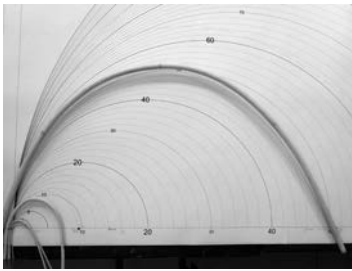
Figure 20,21. Bending radius and member failure as a function of section and pre-stress duration
