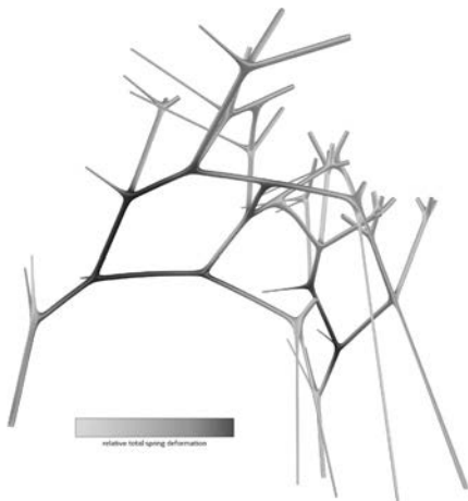
Figure 23a. Localized spring deformation of morphogenetic model due to bending under self-weight during growth
