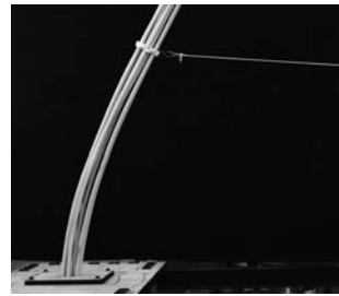
Figure 22. Measuring multiple rattan thicknesses and bundling configurations bending under variable loads
