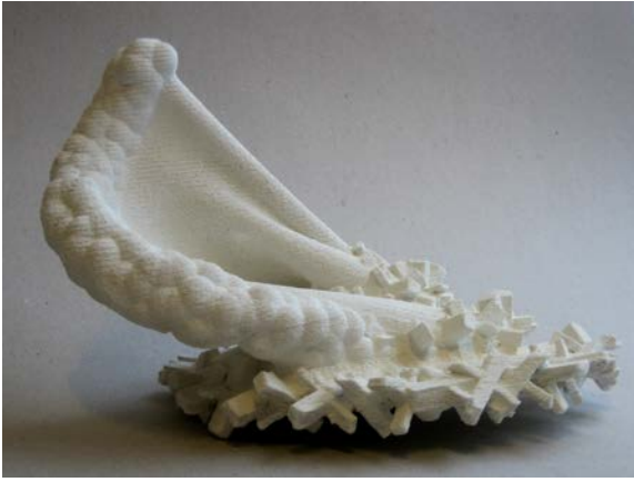
Figure 6: The digital shape is shown as created in ceramics by the use of a 3D powder printer from ZCorp
