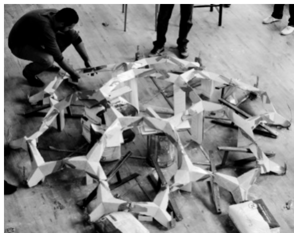
Figure 11: The 'worst-case' prototype after structural failure.
