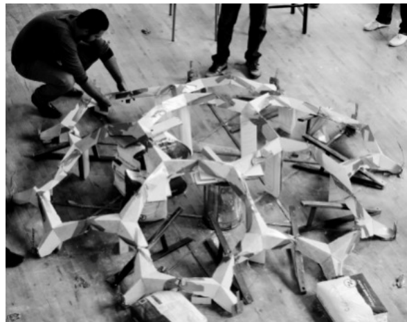
Figure 11: The 'worst-case' prototype after structural failure.
