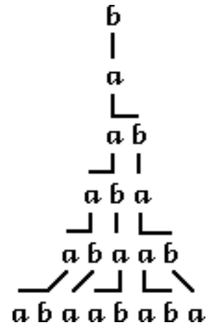
Figure 20: Example of derivation in a DOL-system. The letters are replaced for each generation. Rules: b \rightarrow a , a \rightarrow ab
