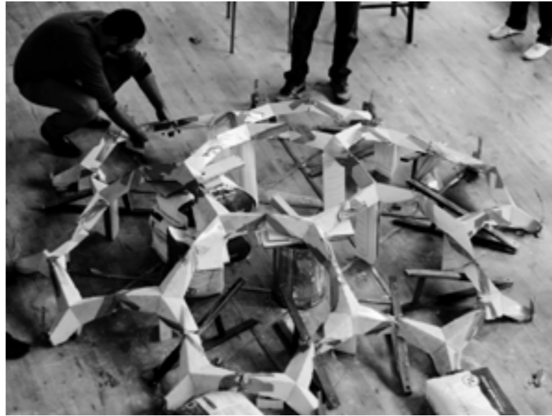
Figure 9: Case study 1. The structure could not be stabilised without connections.
