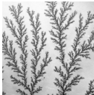
Figure 12: Dendrites of copper crystals. Photo: Pauls Lab
