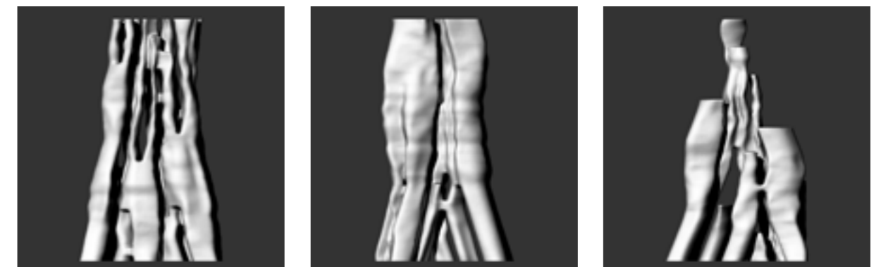
Figure 28: High rise examples. Different versions of floor area control. Left: Reduced area after 800 generations. Middle: Increased area after 800 generations. Right: A 'trunk' growth is stopped at every 200 generations.
