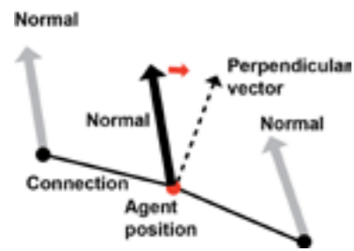
Figure 33. The agent's surface normal is adjusted towards a direction that is an average perpendicular angle to the connection lines.
