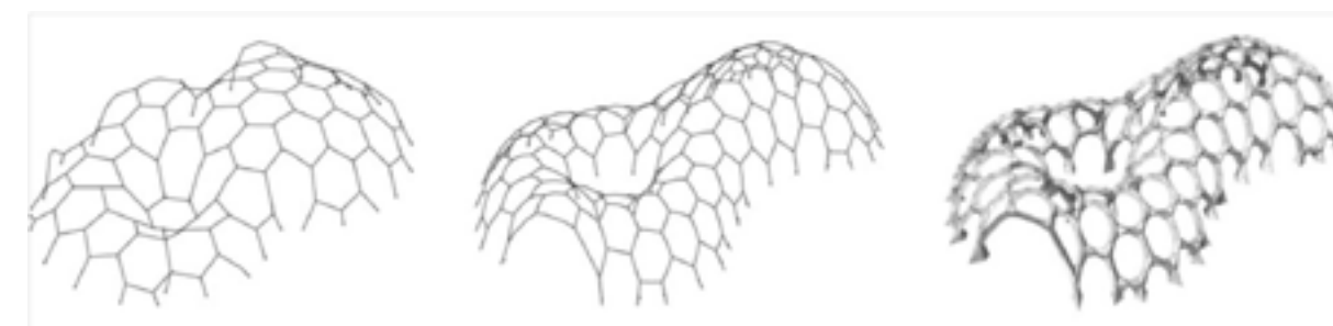
Figure 16: Case study three. Dynamic relaxation procedure and generation of volumetric geometry. Drawings: Ole E. Pedersen.
