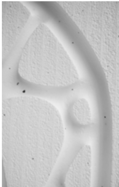
Figure 30: Technological Institute, Copenhagen, Denmark. Images from Digital Crafting workshop, 2010. Left: Polystyrene mould for concrete casting. Right: Robot milling of polystyrene.
