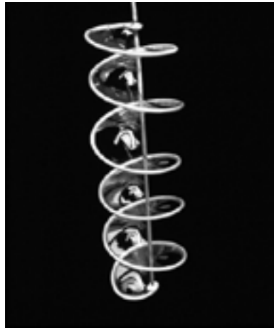
Figure 38. Spiralling minimal surface generated with soap film. Photo: Exploratorium. Middle: A similar shape is achieved with an experiment where the attractor points represent the base geometry of the model. Right: Often, the result would not be a continuous surface.
