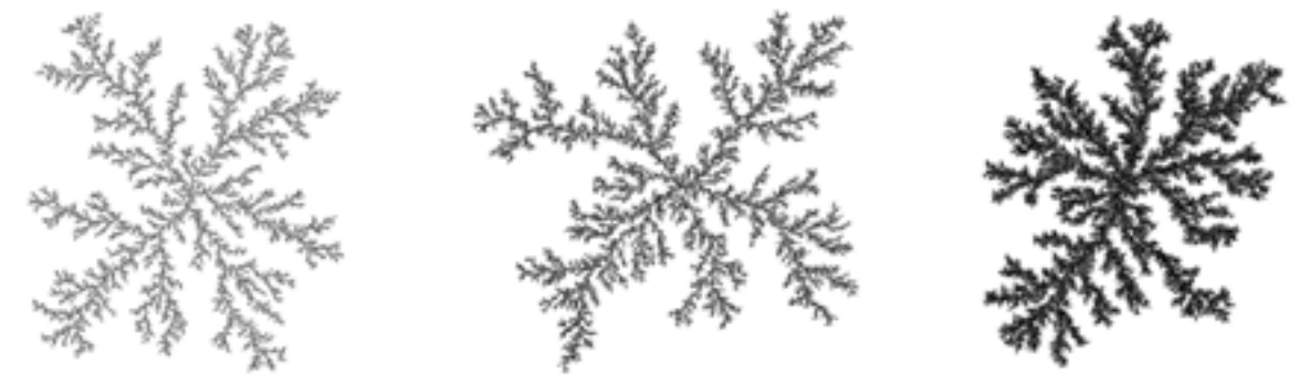
Figure 13: The density of the DLA pattern can be controlled by adjusting the 'stickiness'. The right image shows lowest tendency of sticking. Illustrations by Paul Bourke
