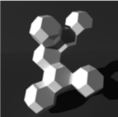
Figure 1: The 14-sided polyhedron was the base component in the experiment. The illustration indicates how identical polyhedrons can be added in 14 different directions.
