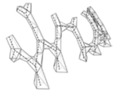
Figure 15: The method Complex Gridshell. Scripting tools serves to generate volumetric geometry and cutting patterns.
