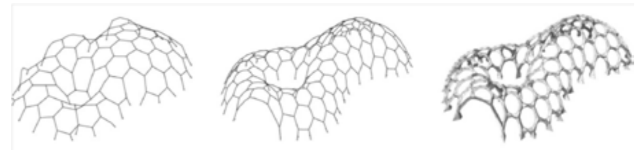
Figure 16: Case study three. Dynamic relaxation procedure and generation of volumetric geometry. Drawings: Ole E. Pedersen.
