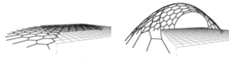
Figure 13: Concrete Gridshell Pavilion, dynamic relaxation simulation. Top: Initial state of the planar mesh. Bottom: Mesh in equilibrium state. Gravity is inverted.
