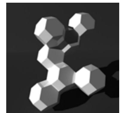
Figure 1: The 14-sided polyhedron was the base component in the experiment. The illustration indicates how identical polyhedrons can be added in 14 different directions.
