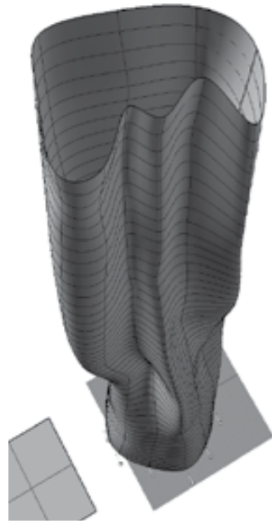
Figure 9. Experiment with a flocking algorithm. The movement of the agents was mapped as control points for constructing a surface.
