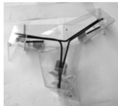
Figure 6: Production of concrete components. Uppermost: Template assembled from laser cut and folded PETG plastic with rebar installed. Bottom: Template with concrete.
