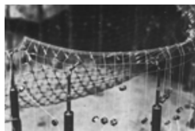
Figure 6: It was possible to adjust the shape of the mesh indirectly by adjusting small weights hanging from the edges of the mesh.
