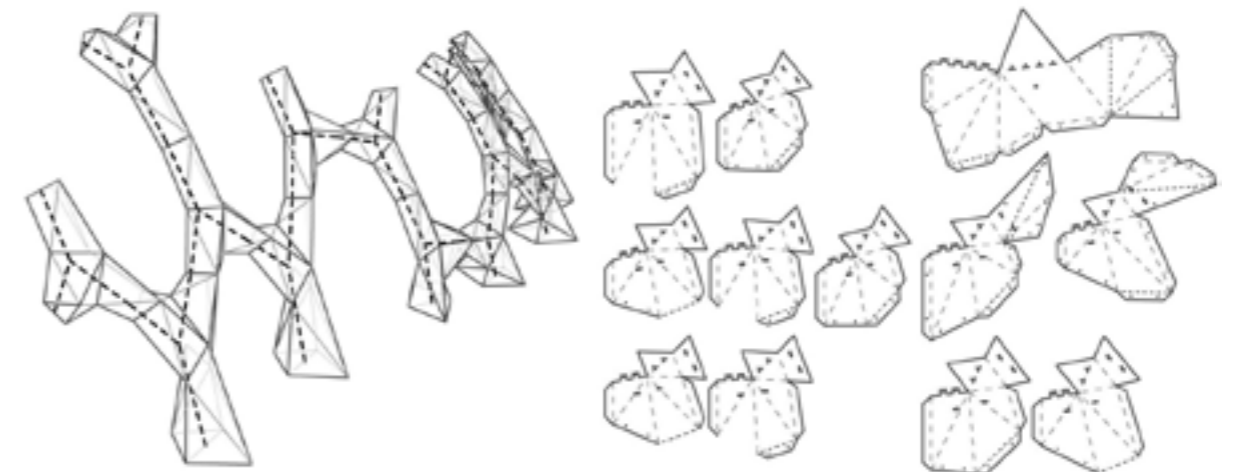
Figure 4: Left: Volumetric geometry, generated from mesh lines. Right: Patterns for laser cutting of templates. Illustration: Dave Pigram.
