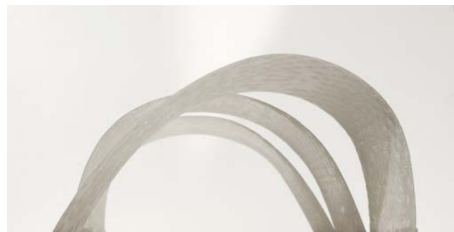
Fig.3 Realised bending behaviour – different responses to the same loading
