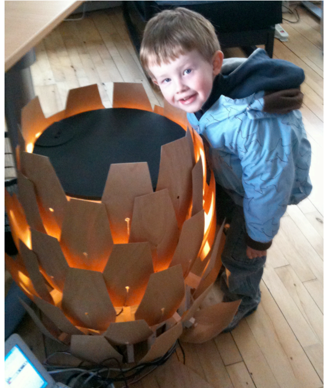
Figure 1. The Home Awareness prototype reproducing light, sound and temperature of a remote place
